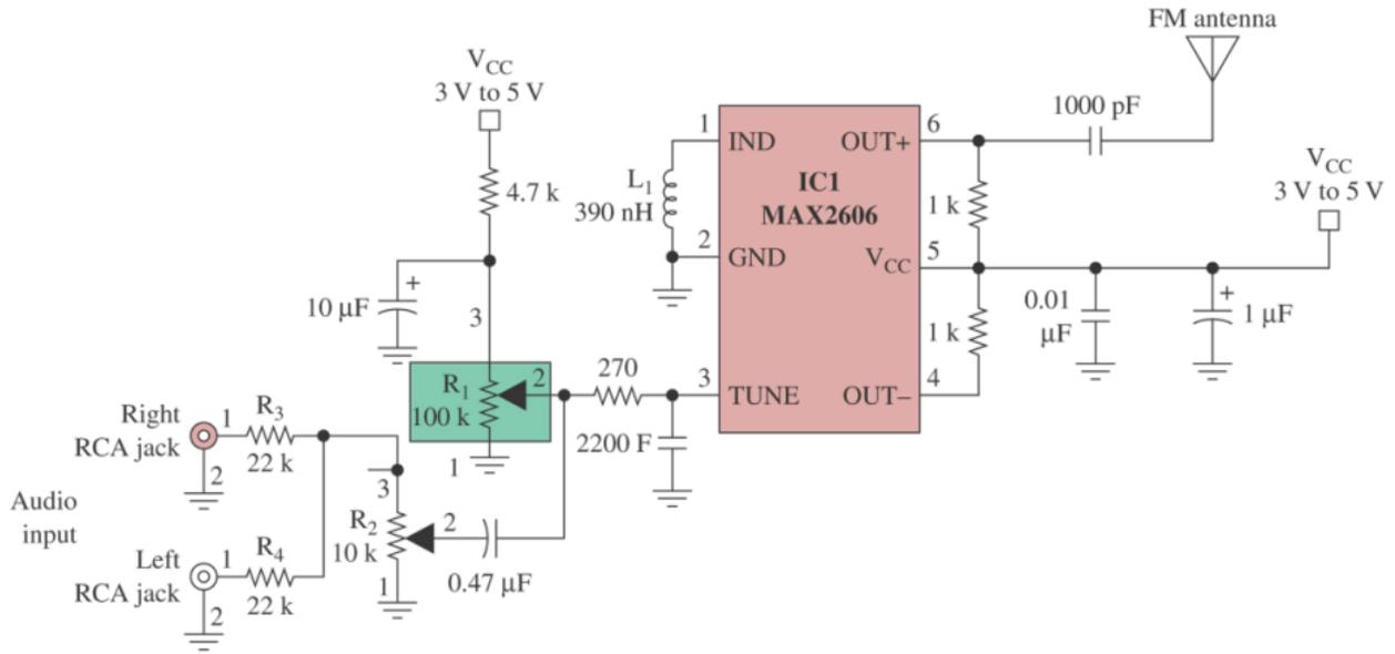
Figure SP8-1 The MAX 2606 single-chip FM transmitter
